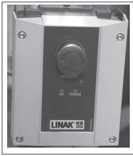
The control box is designed with a red emergency stop and an internal battery charger.
